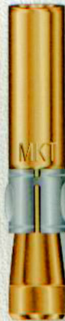
Wedge Anchor B-IG*, internally threaded, steel zinc plated with a supplementary chromate treatment
